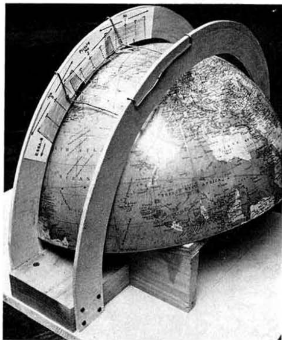
Fig 13. An orbit model for APT satellites in which a half globe can rotate about an axis inclined at about 12^\circ to the vertical plane of the semi-circular strips which mark the limits of view at the sides of the APT picture. The strips are spaced about 30^\circ of longitude measured at the equator. A wire frame is made to scale so that its squares correspond to the fiducial marks on the pictures; its position can be adjusted around the orbit guides. A summer-time sequence for ESSA-8 pictures is illustrated with the wire frame in the No 2 picture position
